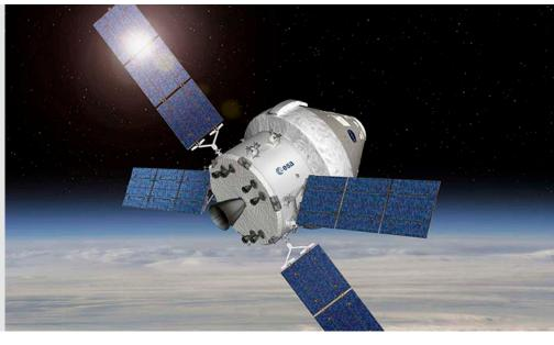
The ESM resembles ESA's Automated Transfer Vehicle, from which it evolved. Between 2009 and 2014, five Automated Transfer Vehicles delivered supplies to the International Space Station and helped to keep the outpost in orbit.
